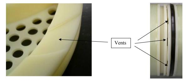
Figure 5: New seal carrier design with recessed vents
