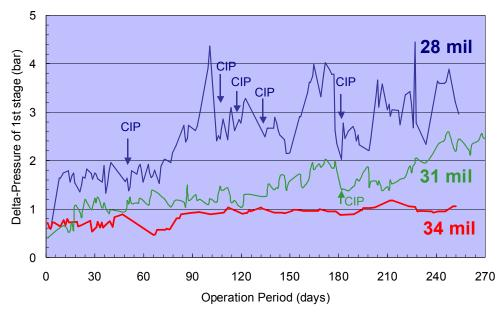
Figure 3: Delta P on surface water feed using different feed /brine spacer thicknesses.
